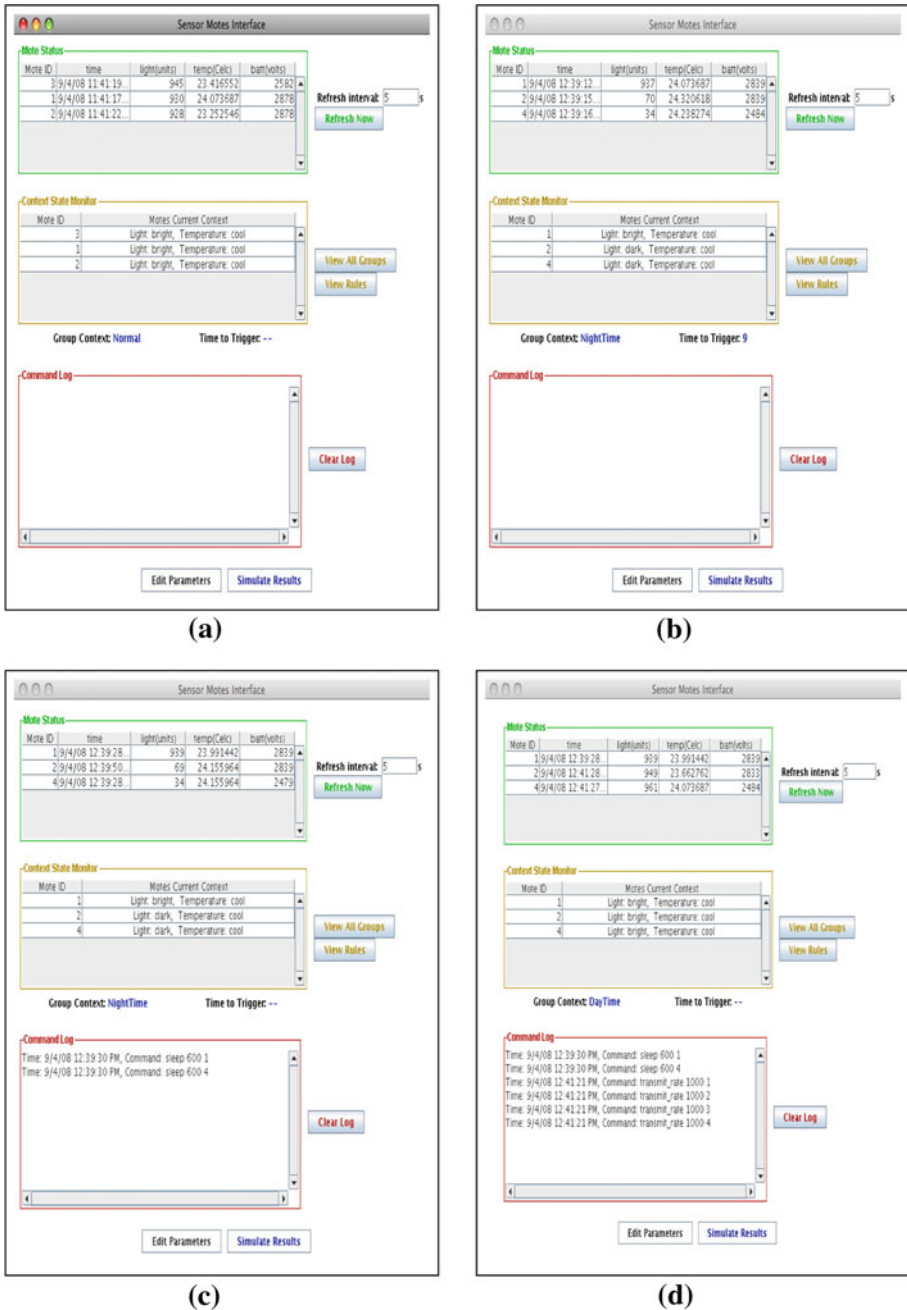
Fig. 16 CASE front-end a Initialisation. b Trigger in process. c Context_tag 'Nighttime' triggered. d Context_tag 'Daytime' triggered
