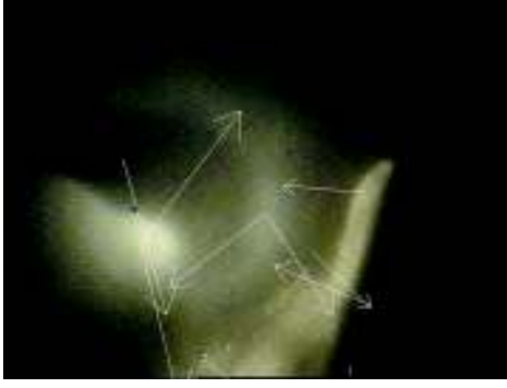
Fig. 5. Detected SIFT keypoints of a flame image.
